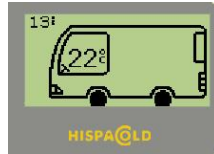
Screen with passenger climatization off
