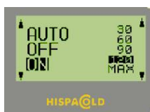
Pre-heater Activation screen.
