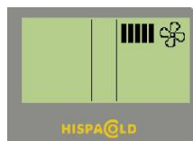
Manual screen (evaporator fans).
